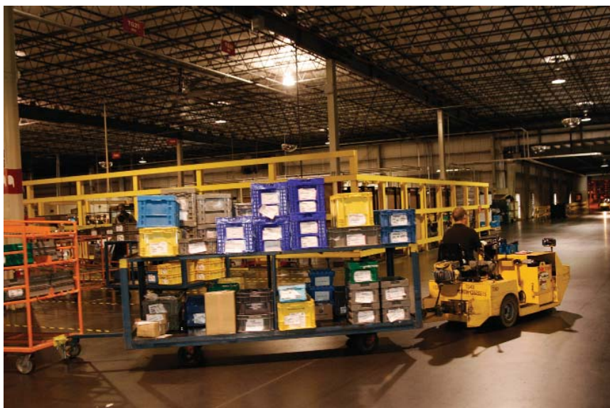
Logistics centers attached to Nissan assembly plants are used to receive, sort, and sequence inbound production parts for delivery to Nissan's vehicle assembly lines.
