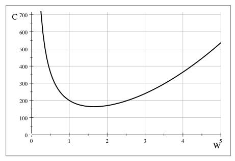
It is clear that the minimum cost does indeed occur when  $W=\sqrt[3]{4.5}$ . The other dimensions will be  $L=2\sqrt[3]{4.5}$  meters and  $H=\frac{5}{\sqrt[3]{20.25}}$  meters.
