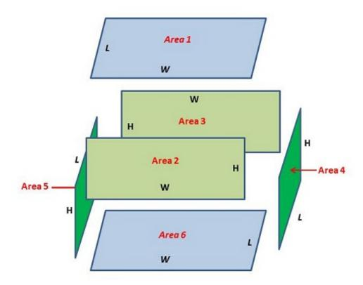
The total cost of manufacturing the box will be the sum of the costs for manufacturing each face. The side faces cost \$6.00 per area unit, while the top and bottom faces cost \$10.00 per area unit. Therefore, our optimization formula will be
