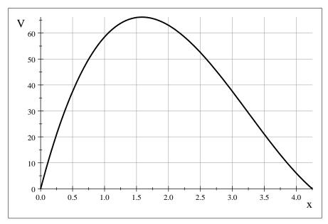
The graph clearly shows that there is a square cutout length that maximizes volume — it appears to be  $x \approx 1.6$  inches. We can use calculus to determine precisely what the value of x should be. Observe that
