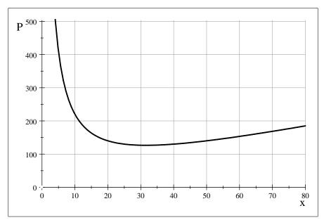
Based on the behavior of the graph shown above along with the fact that we know f has a critical number at  $x \approx 31.62$  tells us that the minimum perimeter does indeed occur when the rectangle has a width of  $x = \sqrt{1000}$  inches. The corresponding length would be
