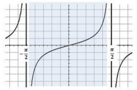
The arctangent function is defined by forming the inverse function for the tangent function on this interval. As with the arcsine function, the arctangent function is defined from its graph. The graph of the arctangent function is obtained by switching the input and output variables for the tangent function on this
