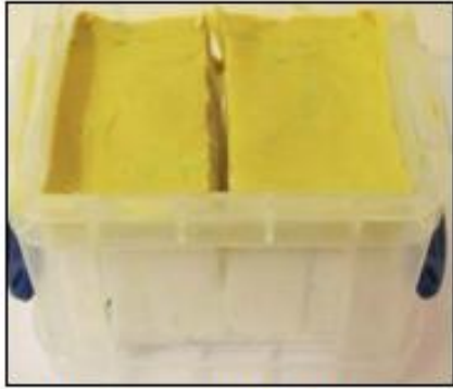
Sugar karst model of a fracture.
